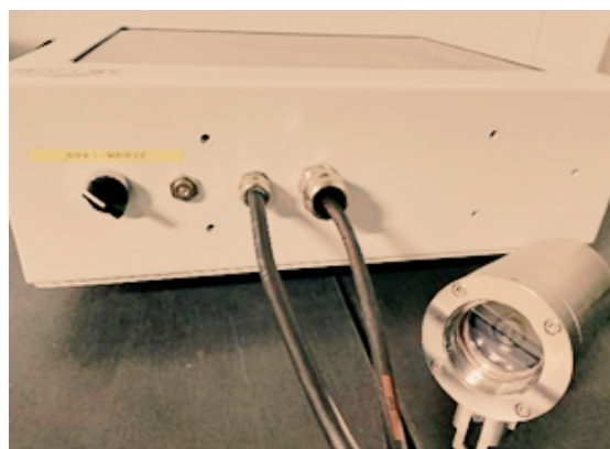
ATEX screen enclosure for a 17-inch display, paired with the ATEX K55 camera and a 20-meter cable.
