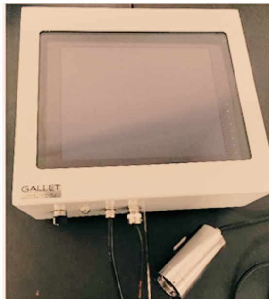
ATEX screen enclosure for a 17-inch display, paired with the ATEX K55 camera and a 20-meter cable.
